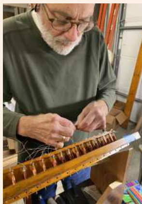
Scott coiling the magnet wires.
