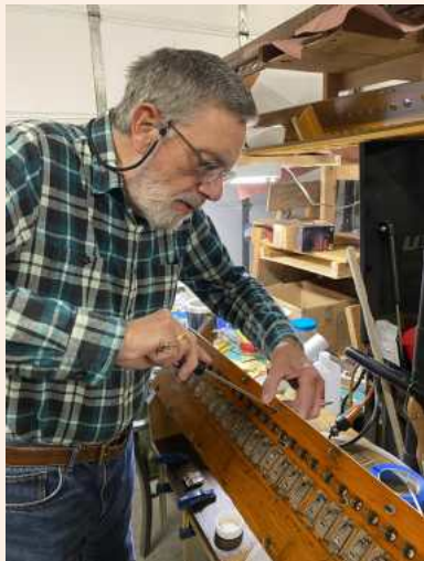
Scott installing a large primary valve guide.
