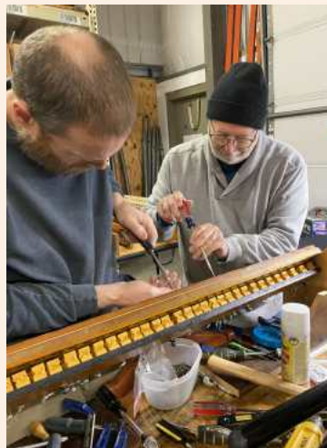
Tim and Brian installing a large primary valve guide.
