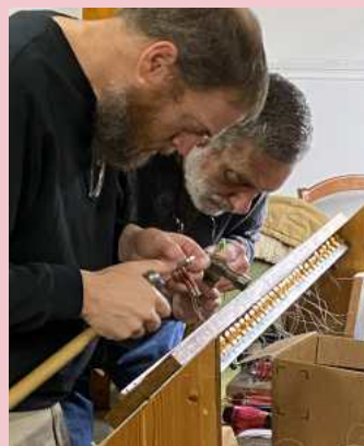
Tim and Scott installing magnets in the bottom board.
