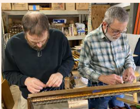
Tim and Scott coiling the magnet wires.
