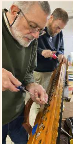
Scott and Tim installing a large primary valve guide.
