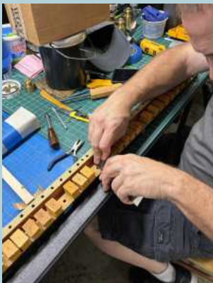
Tim gluing primary pneumatics onto the primary rail.
