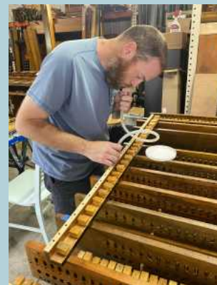
Tim using his personal wind power to test each of the primary pneumatics.
