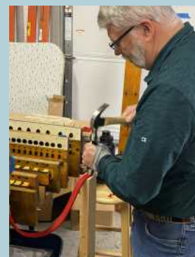
Scott (l) and Brian (r) are punching air holes in some of our custom made gaskets.
