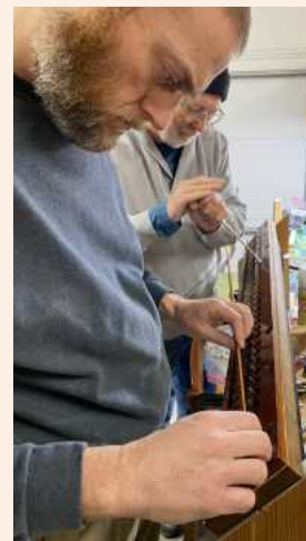
Tim and Brian installing a small primary valve guide.
