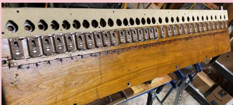
(left) three magnets with cap gaskets installed and three waiting their turn. (below) full bottom board with all magnet cap gaskets installed
