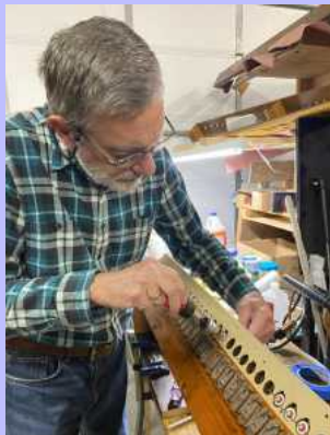
Scott installing primary valves.
