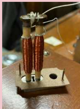
(left) Brian is putting magnet subassemblies together. Right) A completed magnet subassembly.
