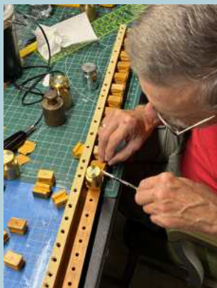
Scott gluing primary pneumatics to the primary rail.
