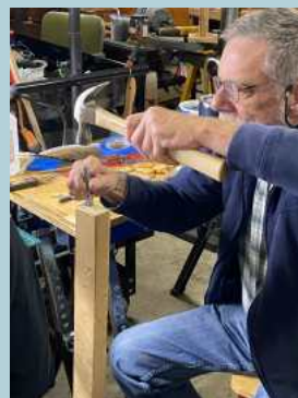
Scott (l) and Brian (r) are punching air holes in some of our custom made gaskets.
