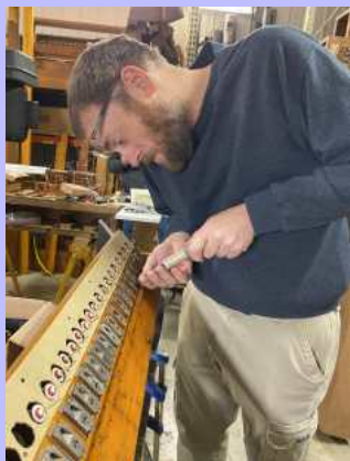
(left) Tim, (center) Scott and (right) Brian. All are working on installing DAG screws which are used to hold the magnet caps in place.
