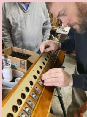
Tim installing magnet cap gaskets
