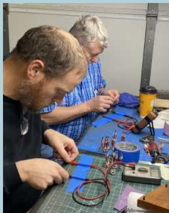
Tim Jones and Brian Hunt doing continuity checks on the magnet coils.
