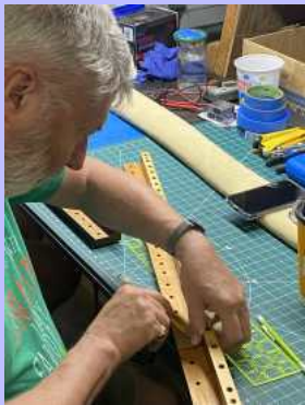
Brian Hunt, Tim Jones and Scott Marsh marking the locations where the primary pneumatics will be located on the primary rail of the bottom boards.
