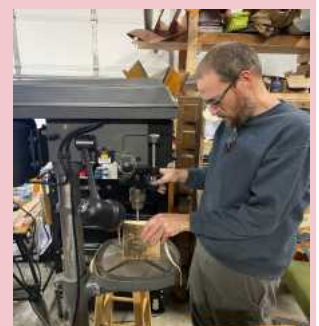
(left) Scott and (right) Tim using the drill press to punch air holes in the gaskets.
