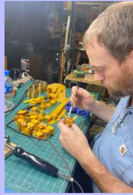
Tim Jones putting glue on the primary pneumatics. This final step seals the air chamber of the pneumatic..
