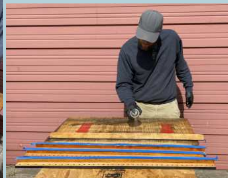
After being cleaned, Tim Jones is applying a coat of shellac to the bottom board wood components.
