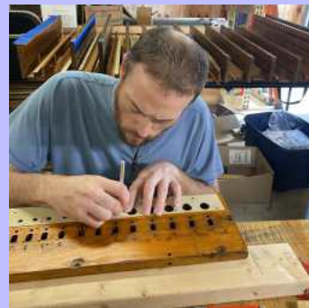
Tim cutting air holes in the gaskets.
