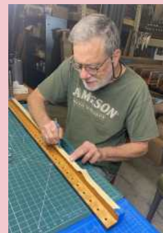
(left) Scott is fitting a gasket to a bottom board rail.
