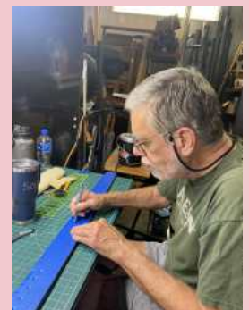
(left) Scott is fitting a gasket to a bottom board rail.
