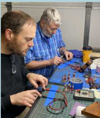
Tim and Brian doing continuity checks on the magnet coils.
