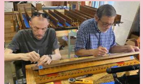
(right) William Webber and Scott Marsh embossing the air holes in the tape mask.
