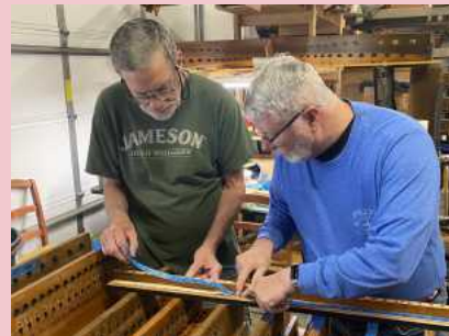
(left) Scott is fitting a gasket to a bottom board rail.
