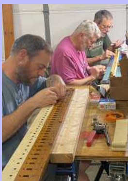
Tim is cutting gasket holes. Brian and Scott are gluing gaskets.
