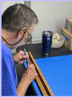
Brian Hunt, Tim Jones and Scott Marsh marking the locations where the primary pneumatics will be located on the primary rail of the bottom boards.
