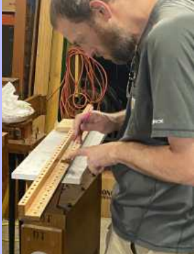
Brian Hunt, Tim Jones and Scott Marsh marking the locations where the primary pneumatics will be located on the primary rail of the bottom boards.
