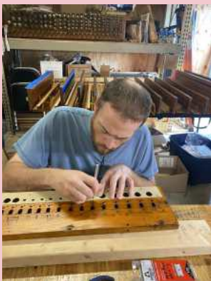
Tim doing some precision cutting of the gasket air holes
