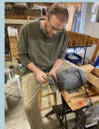
Tim Jones using a wire wheel to do the initial cleaning of a magnet base.
