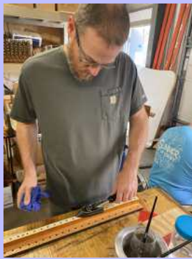
Tim using a heating iron to set the glue on the gasket.
