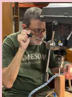
(left) Scott and (right) Tim using the drill press to punch air holes in the gaskets.
