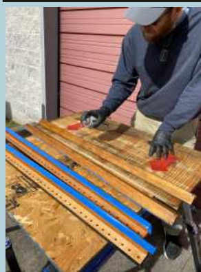
After being cleaned, Tim Jones is applying a coat of shellac to the bottom board wood components.
