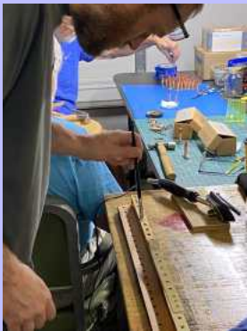
Tim gluing gaskets to the bottom board.
