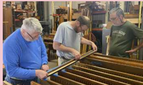
(left) Brian and Tim applying a tape mask to a gasket under Scott's watchful eye.
