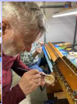
Scott (l) and Brian (r) putting soldering paste on the connecting wires prior to soldering.
