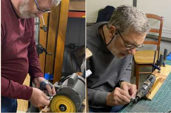
Brian (l) doing the initial polishing of the magnet caps. Scott (r) doing the finish polishing of the magnet caps.
