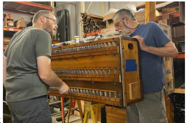
Tim Jones (l) and Scott Marsh next to the 3 rank wind chest with all bottom boards installed.
