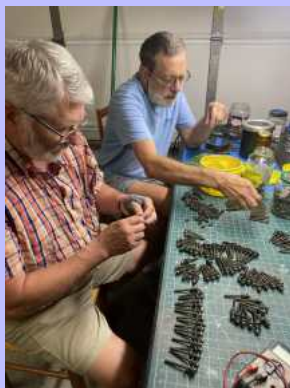
Brian (l) and Scott (r) sorting the screws for the bottom boards. There are two sizes and it is critical to get the right length in the right place.
