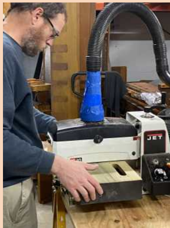
Tim is running the cabinet boards for the Offset chests through a sander to ensure a perfectly flat surface.
