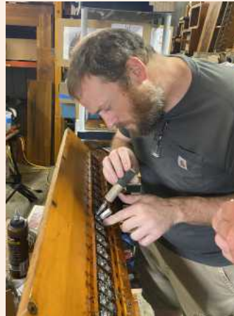
Tim installing the magnet caps
