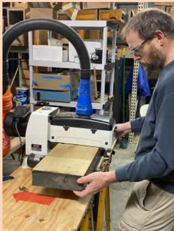
Tim is running the cabinet boards for the Offset chests through a sander to ensure a perfectly flat surface.
