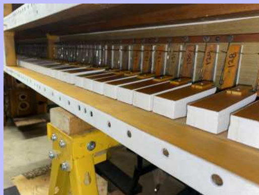
A view inside the 3 rank chest showing the secondary valves (laying horizontally) and the pallet valves (standing vertically). The primary valve on the bottom board will cause the secondary to collapse which will open the pallet valve allowing wind into the pipe creating sound.
