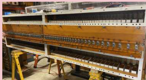
3 Rank Chest with the middle rank (Tibia) installed.
