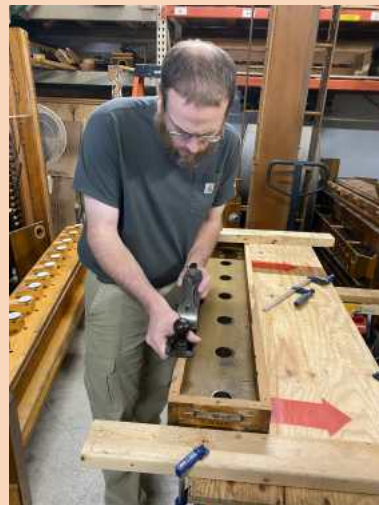
Using a plane to do the final finishing on the offset cabinet boards.
