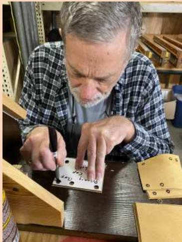
Scott is marking leather gaskets to be used in the offset chests. Each one will be cut out and have the holes punched to match the valves.
