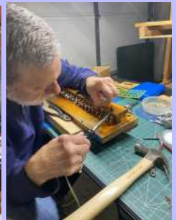
Tim (l) and Scott (r) soldering one of the magnet leads to the common wire which runs the length of the bottom board.
