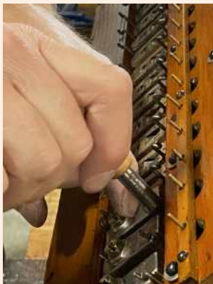
Closeup of the special tool used to tighten the DAG screws which hold the cap on.
