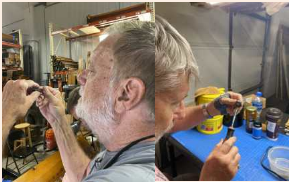
Scott (l) is checking the alignment of the armature in the magnet cap. Brian (r) is adjusting the position of the armature to get it in the right place.
