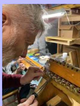
(left) Tim, (center) Scott and (right) Brian. All are working on soldering the other magnet lead wire to the connection which will eventually go to the relay.
