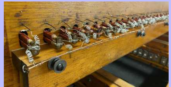
Bottom board with the magnet wires connected.
