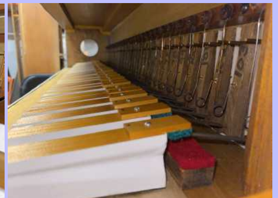
A view inside the 3 rank chest showing the secondary valves (laying horizontally) and the pallet valves (standing vertically). The primary valve on the bottom board will cause the secondary to collapse which will open the pallet valve allowing wind into the pipe creating sound.
