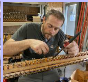
Tim (l) and Scott (r) soldering one of the magnet leads to the common wire which runs the length of the bottom board.
