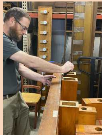
Disassembly of the primary boxes involved delicately prying them apart.
