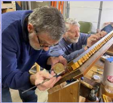
Scott (l) and Brian (r) putting soldering paste on the connecting wires prior to soldering.
