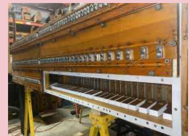
3 Rank Chest with just one board left to install.
