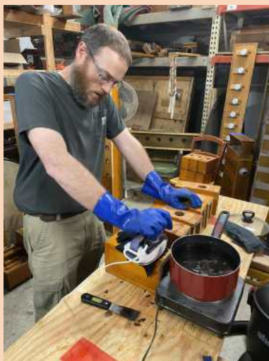
Tim is removing the old gasket material using a hot water bath. The stylish blue gloves were essential.
