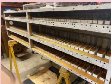
3 Rank Chest waiting for the first bottom board to be installed
