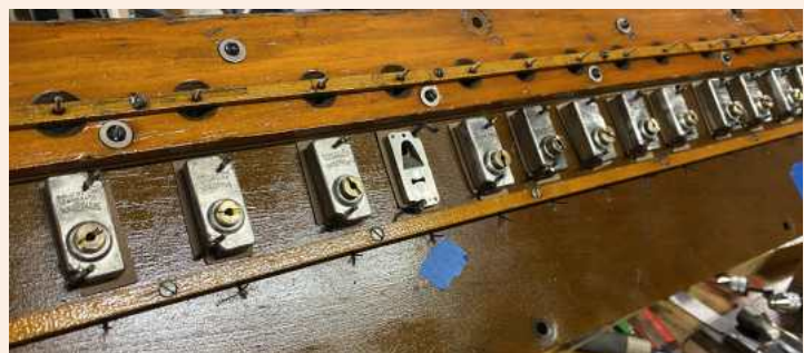
Waiting on one more magnet cap to be installed and this board will be done.
